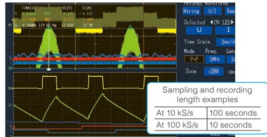
In addition to level triggers, Ver. 3.00 now includes event trigger functions triggered by RMS value and frequency fluctuations. Cursor measurement and waveform zoom functions also render oscilloscopes unnecessary for waveform analysis.
