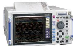
Max. analog 32 channels + logic 32 channels
