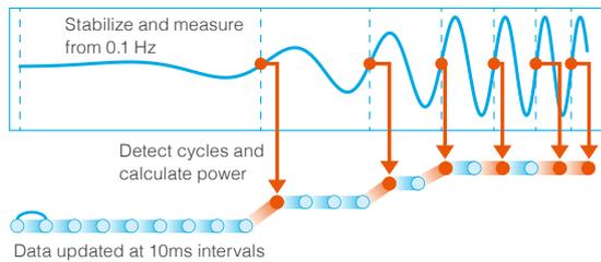
Even during frequency fluctuations from low to high, the fundamental waveform is automatically pursued. Comes equipped with Δ-Y and Y-Δ conversion while calculating with a high degree of accuracy.
